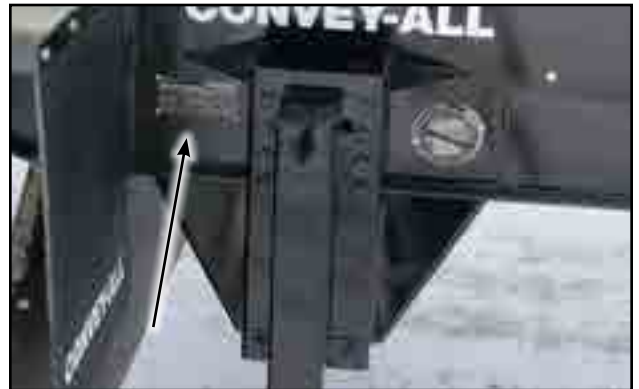
Fig 1 - VIN plate next to front, left-side landing gear
