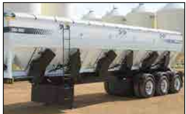
Fig 8 - Exterior ladder brackets
